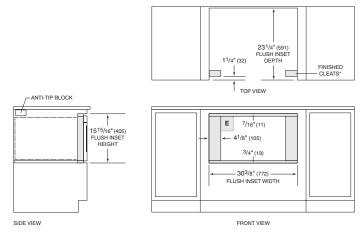
\*Will be visible and should be finished to match cabinetry NOTE: Dashed line represents profile of unit.
