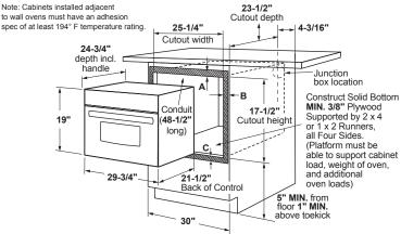
A = The unit overlap is 1/2" but allow 5/8" clearance from top edge of cutout B = The unit overlap is 2-1/4" but allow 2-3/8" clearance from side edges of cutout C = The unit overlap is 1" but allow 1-1/8" clearance from bottom edge of cutout
