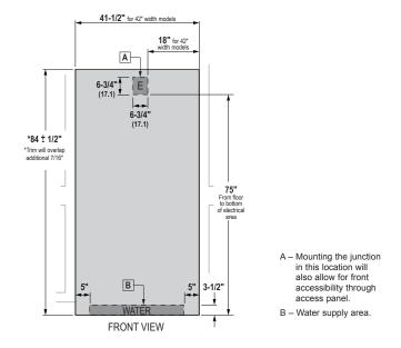
NOTE: GFI (ground fault interrupter) is not recommended. Water line can enter the opening through the floor or rear wall. The water line installed should be 1/4" O.D. copper tubing or GE SmartConnect™ tubing between the cold water line and water connection location. The line should be long enough to extend to the front of the refrigerator. Installation of an easily accessible shutoff valve in the water line is required.
