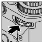
Allows you to set the aperture, shutter speed, and other settings when in [P] / [A] / [S] / [M] modes.
