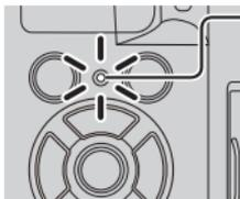
Lit: When the Wi-Fi/Bluetooth function is ON or connected
