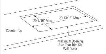
**Note:** If the present opening has rounded corners, the filler pieces should be attached to the straight portion of the cutout. The trim kit will cover any rounded corners.
