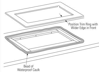
**Note:** A bead of waterproof caulk under the trim ring is recommended. The caulk will prevent moisture or spills from collecting under the trim ring.
