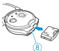
To remove the receiver's battery:
