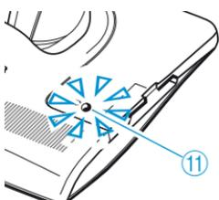
If the operating mode was changed successfully, the charging indicator for the spare rechargeable (11) goes off and the indicator (15) lights up again.
