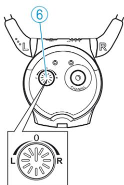
The balance control allows for right/left volume adjustment. Adjust the balance so that you hear equally well with both ears.
