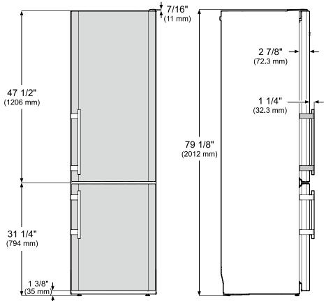
Overall height of the appliance can be increased by a maximum of 5/8" (see Leveling the appliance).
