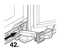
**42.** Slide door cover over soft stop mechanism hinge.
