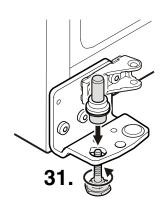
**31.** Tilt appliance slightly backwards, insert pin and attach using the adjustable foot.
