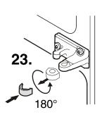
**23.** Remove hinge bushing, turn through 180° and re-fit.
