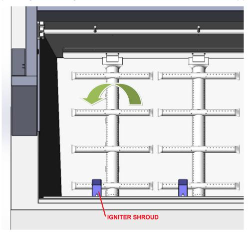
2. You will also need to remove the igniter shroud for the burner you are changing out. Remove both screws shown to reveal the ceramic igniter. The igniter has a perforated sleeve for protection, however it can crack or snap off if you are not careful.
