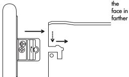
**C.** Insert the Rubber Tabs into the 2 holes on the shorter part of the bracket with the flat side facing up.
