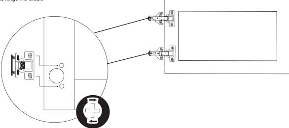
Note: The hinge can be separated by pulling the black tab and pulling apart the hinge from the hinge base.
