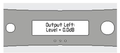
Once selected the volume level will appear on the display. Use the dial to change the volume level (from -60dB to +12dB) and press the dial once again to confirm the volume level selection. The display will start with the Left Output, then to the Right Output, and lastly to the Sub Output. To return to the "Change Volume" page, press the dial again. To exit the menu, select "Exit Menu" and press the dial.
