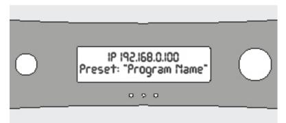
Turn the dial to select your desired preset to match your Origin Acoustics Speakers. If you are not sure which preset to use, refer to the "Amplifier Preset" section of this manual. Once you have found the desired program number it will be blinking. Press the dial to select the desired program to load, at which time it will stop blinking. If the number is not blinking while selecting, the display will return to the "Load Program" menu and you will need to restart the process.
