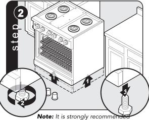
that a pallet or lift jack be used rather than tilting. Raise unit about a foot. Unscrew shipping bolts from couplings on all four corners.
