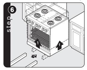
Lift unit and prop on wood blocks.
