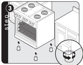
Screw legs into couplings on all four corners. The 48" W. ranges have two additional legs located in the center of
