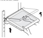
**3** To assemble, tilt the front of the shelf up and guide the shelf hooks into the slots at a desired height.
