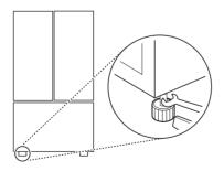
Open both doors and check to make sure that they close easily. If the doors do not close easily, tilt the refrigerator slightly more to the rear by turning both leveling legs to the left. It
