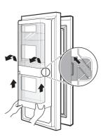
Pull out the crisper to full extension, lift the front up, and pull straight out.
