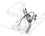
4 Push the water supply tube into the hole on the top case and pull it through the backplate.
