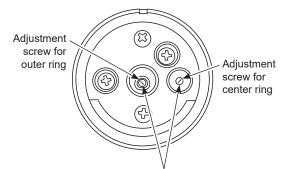
Adjustment screws for multi-ring burner only
