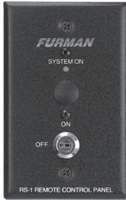
The RS-1 features a two-position key operated switch, an indicator LED, and can be easily installed in any electrical switch box with a minimum depth of 1-1/4". On the rear is a printed circuit board with a standard size terminal strip for wiring connections.
