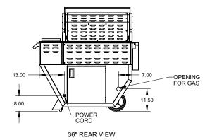
GAS REQUIREMENTS: 1/2" NPT gas connection. Minimum gas supply is 7" water column for natural gas and 11" for propane. Operating pressure at the manifold is 4" water column for natural gas and 10" for propane. All units require a regulated gas supply. (included)
