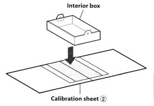
(2) Line up with the center line on calibration sheet ② and draw a center line on the interior box.
