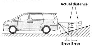
The distance guidelines represents the distance to a flat road surface. Therefore in the case of an upward slope behind the car, the distance guidelines appear further from the vehicle than their actual position. For example, if there is an object on the upward slope, it may appear further away than its actual position.
