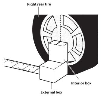
Align the center line of the interior box with the center of the tire.
