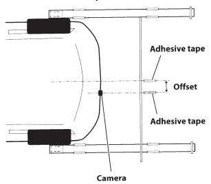
Place calibration sheet ② on the ground so that the sheet center line aligns with the offset spot marked in step 6, and affix calibration sheet ② to the ground with adhesive tape so it is parallel with the measuring tape.
