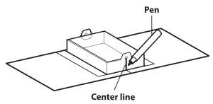
2 Affix the calibration sheets ① on the ground so they align with the vehicle width.
