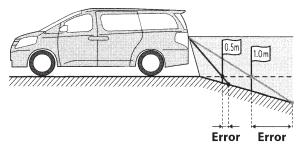
In the case of a downward slope behind the car, the distance guidelines will appear further away than the actual distance. If there is an object on the downward slope, it may appear closer than its actual position. Also, an error may occur between the guidance and the actual path of the car on the road surface.
