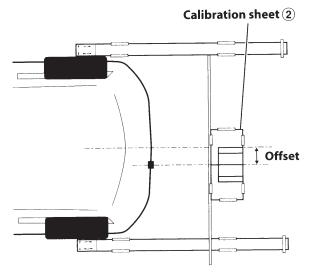
Make sure that the measuring tape lines up with the measure mark values, and are the same for both the left and right calibration sheets.
