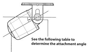
Install the camera so that this rounded part is clearly visible then viewed from the side of the vehicle.
