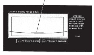
Adjust so that the bumper appears within the orange adjustment frame. The bumper should take up about 10% of the area inside the frame.
