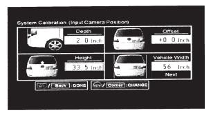
You can specify the height from the ground to the camera in 0.5 inch/1 cm increments by pressing SET..
