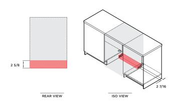
Service outlet at rear extends both sides, hoses and cords can be routed to either or both sides
