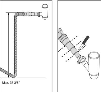
The drain hose can also be connected to a connection nipple on the sink's water trap. The connection nipple must have an internal diameter of at least 1/2". The water trap must be ventilated.
