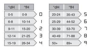
Do not forget to put salt in the salt compartment after you have set the water softener to 1 - 9.
