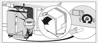
4 Adjust the front feet by turning them clockwise to raise and counterclockwise to lower the dishwasher.
