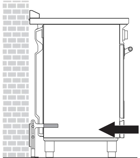
10. Check for proper installation and use of the anti-tip bracket. Carefully tip the range forward by pulling it from the back to ensure that the anti-tip bracket engages the range leg and prevents tip-over. The range should not move more than 1" (2.5cm).
