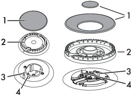
2. Unscrew the burner nozzles using a 7 mm socket wrench;
