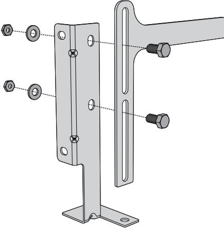
3. Align the base of the hook of the bracket with the base on the slot of the rear wall fastening bracket. Align the base of the fastening bracket with the floor and tighten the screws to fix the measurements.
