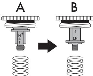
4. Screw the regulator stem and cap into place.
