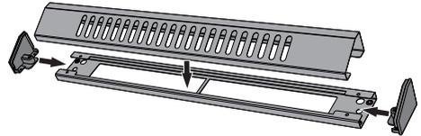
2. Position the backguard above the top, taking care to align the holes.
