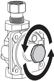
2. Unscrew the plastic regulator stem from the regulator cap. Configuration "A" is for Natural Gas.
