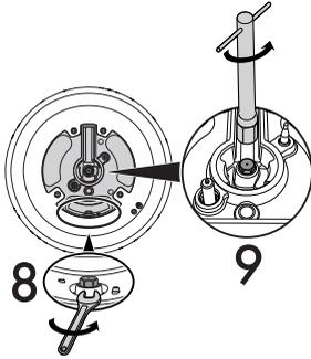
3. Refit the burner components correctly.
