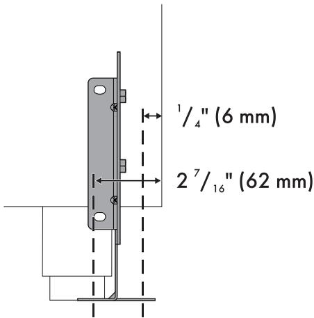
8. After having positioned and leveled the appliance, move the bracket close to the rear of the appliance and anchor it to the floor using the two washers and screws. A qualified technician must verify the suitability of the materials in accordance with the type and condition of the floor.
