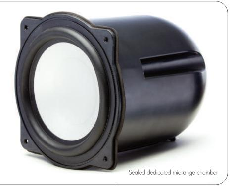
• Sonic Solidarity! A sealed chamber behind the dedicated midrange driver, made of GRIP™ glass-reinforced injection-molded polymer. The design prevents the massive air pressure generated by the woofer from coloring sound output.
