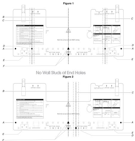
**NOTE:** If wall studs is within 6" (15.2 cm) of the vertical centerline (see "Mark Rear Wall" section), only recirculation or roof venting installation can be done.
