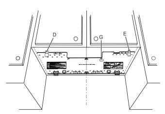
**Note:** If upper cabinet is metal, the supply cord bushing needs to be installed around the supply cord hole as shown.
