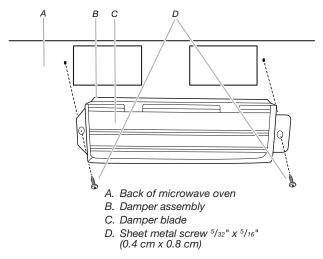
3. Secure damper assembly with 2 Sheet metal screws  $_{^{5}\!/_{32}"}$  x  $_{^{5}\!/_{16}"}$  (0.4 cm x 0.8 cm)
