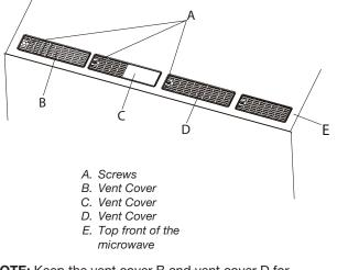
**NOTE:** Keep the vent cover B and vent cover D for recirculation in future.
