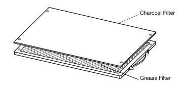
Vent Cover Installation (for both upper vent and wall vent installation)
