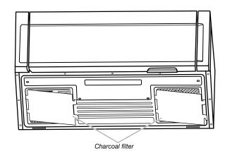
**3.** Replace a new charcoal filter and reattach it back to the bottom plate, and make sure both left and right sides insert into the bottom plate slots.
