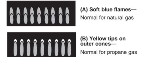
Long, bright yellow flames are not normal. Normal flames may show signs of an orange tint when well heated or signs of flickering orange due to particles in the gas or air.
