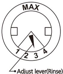
Turn the rinse aid indicator dial to a number between 1 and 4. The higher the number, the more rinse aid the dishwasher uses. If the dishes are not drying properly or are spotted, adjust the dial to the next higher number until your dishes are spot-free. Reduce it if there are sticky whitish stains on your dishes or a bluish film on glassware or knife blades.
