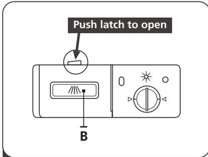
**1** Press the release catch on the detergent dispenser to open the cover.
