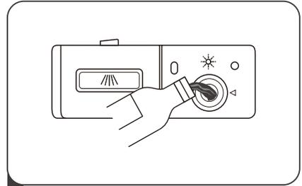
**2** Carefully pour in the rinse-aid into its dispenser, whilst avoiding it to overflow.
