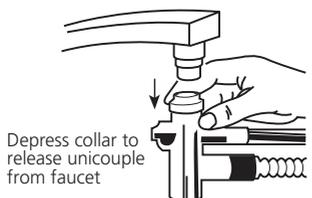
3. Depress the locking collar and remove the uncoupler from the faucet.
