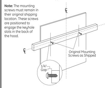
• Adjust depth of original mounting screws in the wood support until they protrude 1/4" forward. This 1/4" gap will provide clearance to hang the hood.
