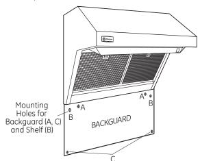
• If installing the backguard alone, without the shelf, drive screws in all locations shown.
