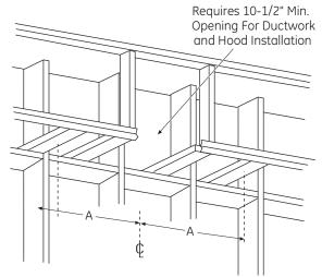
• The 2 x 4 studs must be located as shown in the chart, Dim. A. to accept mounting screws.
