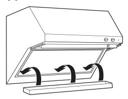
• Insert the grease filter into the opening and drop into the bottom. Raise filter to the top and lock into place.
