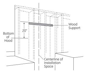
• Secure the wood support to 2 or more vertical studs, using at least 2 of the 4 supplied long screws.
