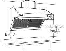
• From the line indicating the bottom of the hood, measure 20" up and draw another line for the location of the wood support. See illustration.
