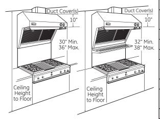
**Note:** When determining the installation height, consideration must be given to the use of the warming shelf.
