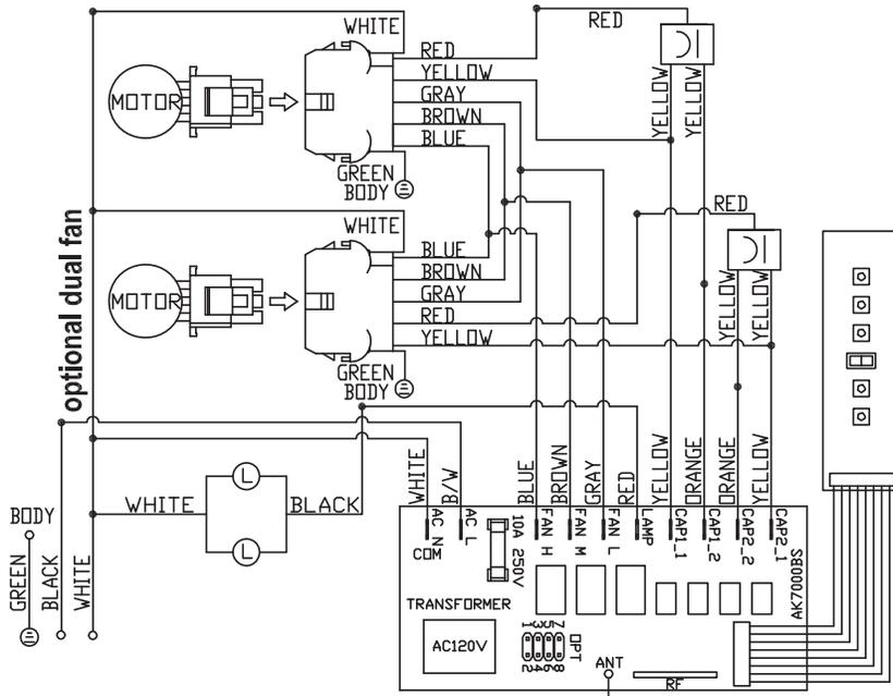
REMARKS: CONDENSER 11+11uF 250VAC 2PCS FIT AC120V 60Hz
