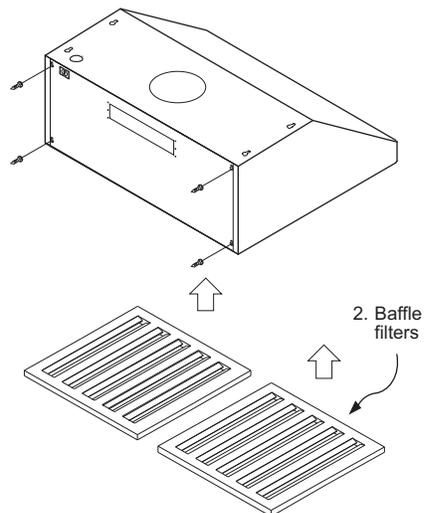
This range hood is equipped standard with a 8" round vertical duct option. To convert from 8" round vertical to 8" round horizontal ducting or 3-1/4" x 10" rectangular horizontal ducting please following the instructions below.
