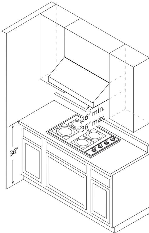
Minimum mount height between range top to hood bottom should be no less than 26".
