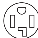
4-Wire Receptacle (14-30R)
