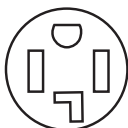
4-Wire Receptacle (14-30R)
