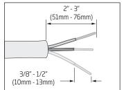
Electrical supply cords must be a minimum #14AWG copper wire. The dishwasher is designed for an electrical supply of 120 V, 60 Hz, AC, connected to a dedicated, properly grounded electrical circuit with a fuse or breaker rated for 15 amperes.
