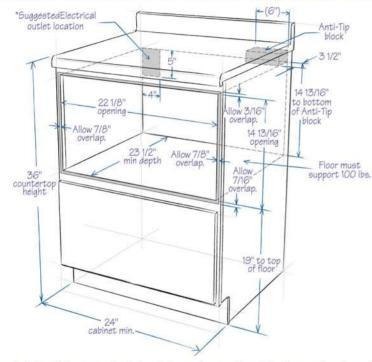
\* Can also be installed using an electrical outlet in an adjacent cabinet within the area where the provided electrical cord can reach. Power cord access hole in cabinet should be a minimum 11/2" diameter hole and deburred of all sharp edges.
