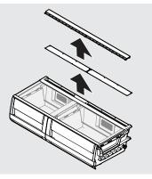
Removing Auto Humidity Control Membrane
