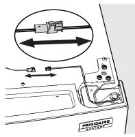
5. Pull up on water line gently to remove from door.
