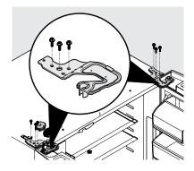
In certain circumstances, you may need to remove the lower hinges for clearance purposes. To gain access to the lower hinges, first extend the Custom-Flex Temp Drawer. Unscrew the 3 lower hinge screws and slide the hinge inward.
