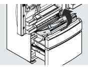
Unsnap the 4 cable ties by pressing clip sides together and pushing them through the opening.
