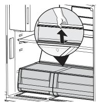
Removing Auto Humidity Control Membrane
