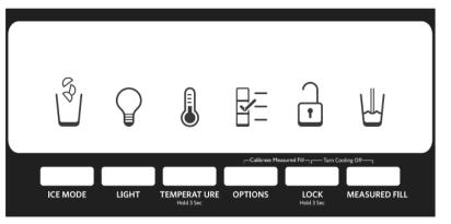
For your convenience, your refrigerator and freezer controls are preset at the factory. When you first install your refrigerator, make sure that the both the refrigerator and freezer controls are still set to the "mid-setting." This will be indicated with three illuminated bars.
