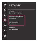
4 The device automatically tries to connect to the available network (wired network first). When you select the Wi-Fi Connection, the network list available is displayed. Choose the network you wish to use. For wireless AP (Router) that has the symbol, you need to enter the security key.
