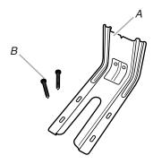
A. Anti-tip bracket B. #12 x 1 5/8" screws (2)
