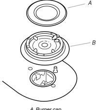
A. Burner cap B. Burner
