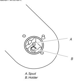
**NOTE:** This range is equipped with 2 standard burners and 2 super burners. Spud size and location remain the same.
