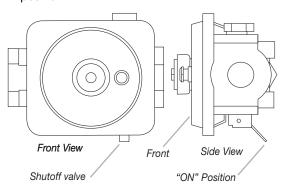
**3.** Open the manual shutoff valve in the gas supply line. The valve is open when the handle is parallel to the gas pipe.
