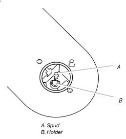
**NOTE:** This range cooktop is equipped with 2 standard burners and 2 super burners. Spud size and location remain the same.
