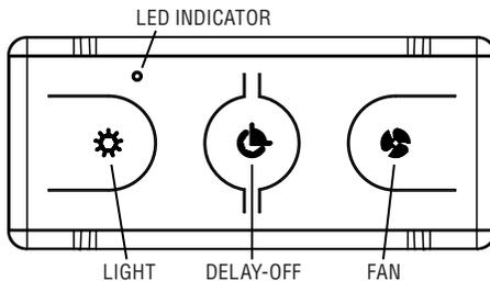
**Light Button** – When the hood lights are OFF, pressing the light button will turn the hood lights ON to the lowest setting. Pressing again will index the lights to the next highest setting. When lights are at the highest setting, pressing the button again will turn lights OFF.
