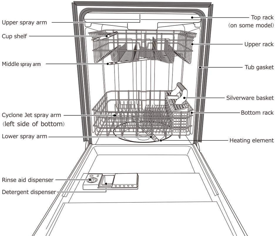
Remark: The picture only shows the position of each parts. There are differences between the parts of different models. Please refer to the actual parts.
