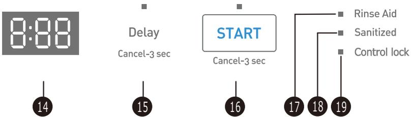
**14 - Display**—Shows the remaining hours and minutes of the current cycle, delay hours remaining, and error codes (see “Error codes” on page 27).
