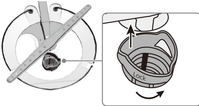
3 Lift the fine filter from the bottom of the tub.
