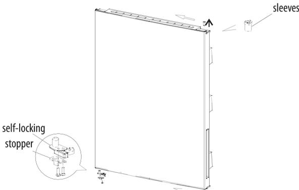
6) Remove the center hinge, remove the center hinge shaft with a slotted screwdriver, install hinge shaft on opposite side of the hinge and install the hinge to the left of the box.
