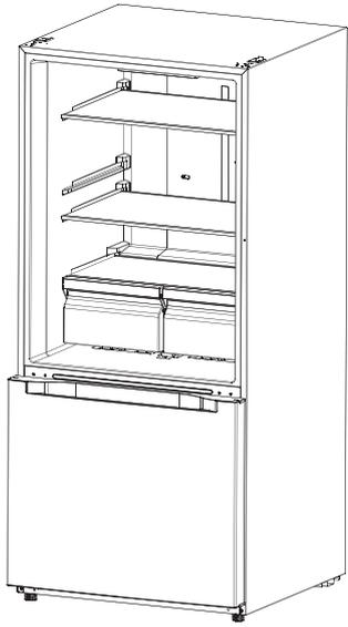
7) Put down the refrigerator door on the middle hinge vertically, then take out the top hinge and cover of other side from accessory bag, assemble top hinge, hinge cover and hole cover.
