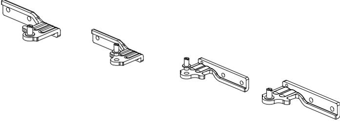
In the order shown above, the center hinge shaft is changed.
