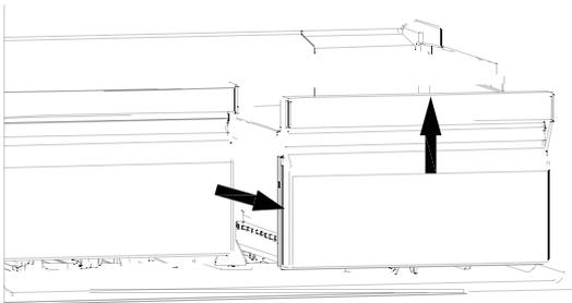
2. The roller seat is stuck in the box tank groove, press the arrow in the direction of the image, remove the roller seat, clean the box tank groove as needed.
