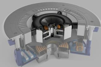
Cavity Radiation Control is a unique open-back midrange with acoustically absorptive foam design that eliminates midrange distortion, up to 30dB midrange dip, found in typical coaxially arranged three-way designs. Cavity Radiation Control enables KEF coaxial three-way architectural speakers to deliver the highest midrange acoustic realism.
