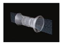
After – Turbulence has been significantly reduced in the bookshelf speakers' CFD-designed ports
