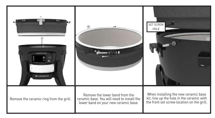
Install the bands and attachments on your new ceramic base. Repeat the steps in reverse order to install the new ceramic base kit.
