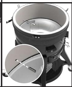
Remove the set screw from the inside of the grill (front).
