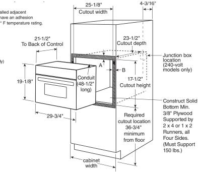
A=Allow 1" overlap of oven over bottom edge of cutout. B=Allow 11/16"-3/4" for overlap of oven over side edges of cutout.
