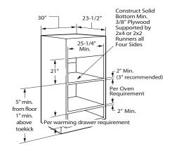
\* For existing cutouts, a maximum width of 28-1/2" is acceptable. If the opening is slightly wider, secure a furring strip on each side of the cutout for securing the oven.
