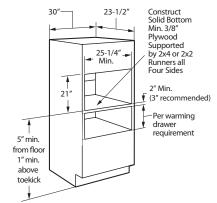
\* For existing cutouts, a maximum width of 28-1/2" is acceptable. If the opening is slightly wider, secure a furring strip on each side of the cutout for securing the oven.
