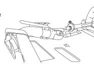
4. With a 1/2" wrench, loosen each orifice by turning counterclockwise and remove.
