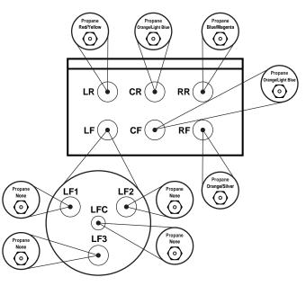
To prevent leakage, make sure the orifice spuds are securely screwed into the gas supply tubes.
