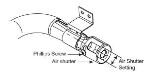
With a Phillips head screwdriver, loosen the screws securing the air shutters on the burners and adjust the air shutters according to chart above.
