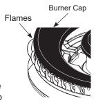
E. Additionally, for each burner being adjusted, quickly open and close the oven door while observing flame. If flame is extinguished, continue adjusting bypass screw for a larger flame. Repeat door openings until flame is stable.
