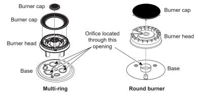
B. Using a 7 mm or 9/32" nut driver, remove the top burner orifices. These may be accessed through the burner opening in the base.
