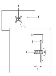
A: Wall Mount Plate B: Back of the Monitor C: Standard screw D: Max. 8 mm (0.3 inches)
