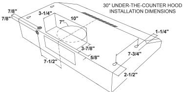
Exhaust outlet connects to 3-1/4" x 10" rectangular duct. Vent top or rear. Includes rectangular damper.
