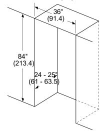
Leave 1/2" gap at the top and 1" behind the refrigerator for proper ventilation.
