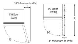
Allow 4-1/2" min. clearance on the hinge side for the 90° door swing and to allow racks to slide out.
