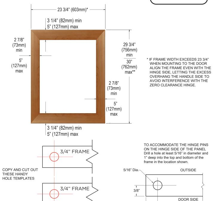
AFTER INSTALLATION UNDERCOUNTER, OVERLAY DOOR MUST BE ABLE TO OPEN 90°.
