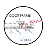
7 Using the (10) ST4-30 self-tapping screws supplied securely fasten the frame to the door. Do not over tighten as screws may strip out. WARNING: Screws are sized for 3/4" panel, DO NOT USE these screws for thinner panels.
