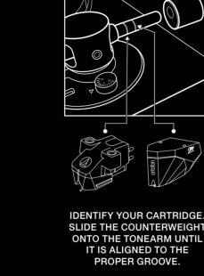
PROPER GROOVE **ORTOFON 2M SERIES** COUNTERWEIGHT SLIDES TO THE FIRST GROOVE
