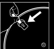
CAREFULLY REMOVE THE TAPED GUIDE STRING AND PULL THE BELT OVER THE MOTOR PIN. DISCARD THE GUIDE STRING.
