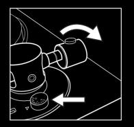
ONCE ALIGNED WITH THE CORRECT GROOVE, TURN THE TOP SCREW CLOCKWISE TO TIGHTEN THE COUNTERWEIGHT
