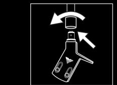
INSERT THE HEADSHELL INTO THE TONEARM AND TIGHTEN THE TONEARM COLLAR COUNTER-CLOCKWISE UNTIL HEADSHELL IS SECURE.
