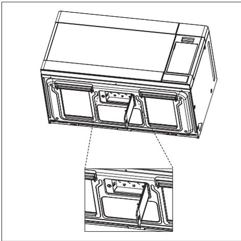
2. Remove the vent grille mounting 3 screws and open the door.
