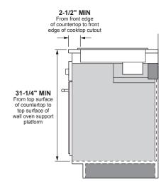
Dimension and installation information are shown in inches. \*Allow 5-3/4" depth at rear for electrical and gas connections
